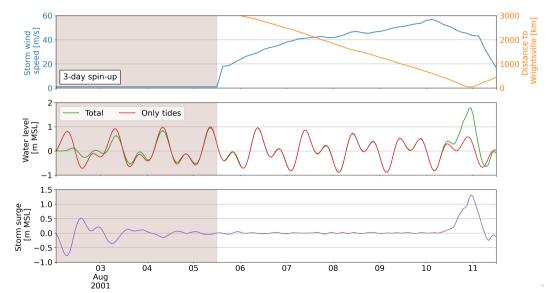
**Step 2:** Hydrodynamic modeling with ADCIRC Storm 0 – Time series at Duck NOAA tide gauge
