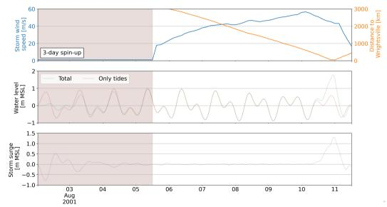
**Step 2:** Hydrodynamic modeling with ADCIRC Storm 0 – Time series at Wrightsville NOAA tide gauge
