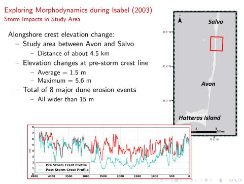
Initial Results with XBeach Generating Mesh for XBeach Simulations
